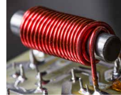
Fixing and securing of ferrites in air coils
