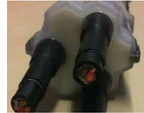
Sealing of cable bushings and housings
