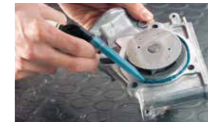
Project: Sealing of pump with silicone
