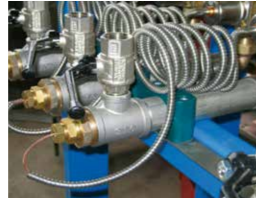
Bonding and sealing of pipe threads
