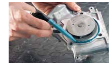
Project: Sealing of pump with silicone
